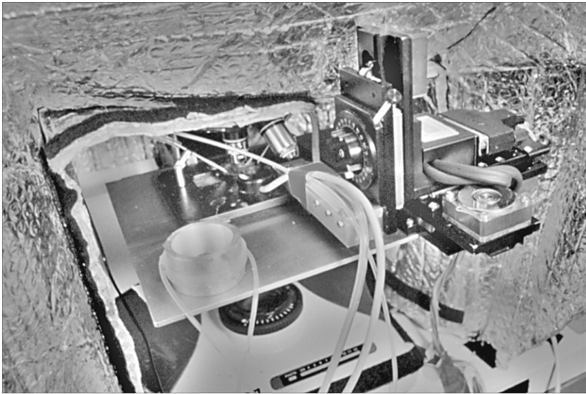
Fig. 4. The RoboStage, consisting of a Sutter MP-285 micromanipulator, is connected via the serial port to the computer that controls the 2-photon microscope. This view inside the environmental enclosure shows the culture dish holder bolted to the manipulator, which is in turn bolted to the stage of the microscope. The manipulator is programmed to move the specimen to several fields of view, repeatedly, in sequence, under the stationary objective lens. A perfusion system keeps the medium in the culture fresh and allows pharmacological manipulation of the network during time-lapse imaging.
